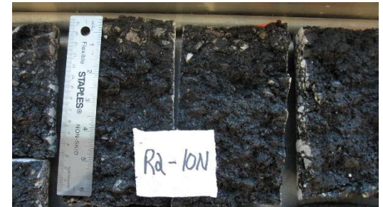
Cores heated to \sim 60^{\circ}\text{C} , split in lab; moisture damage rated L, M, H severity
