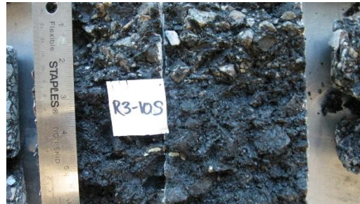
Cores heated to \sim 60^{\circ}\text{C} , split in lab; moisture damage rated L, M, H severity
