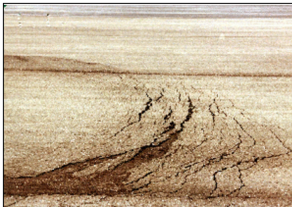
Distortion - High Severity (With Associated Tear Cracking)
