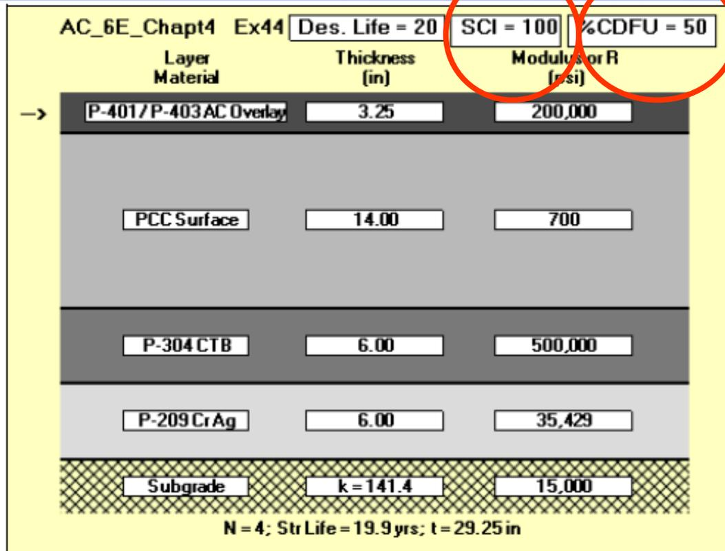
Use SCI 100 for good pavement and heavier aircraft or after repair of distressed slabs
