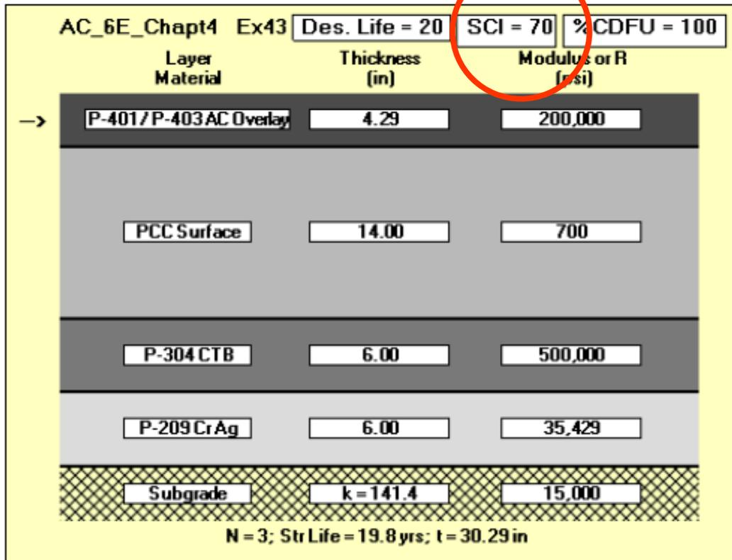
FAARFIELD iterates with base and overlay deteriorating at same rate until design life is achieved.
