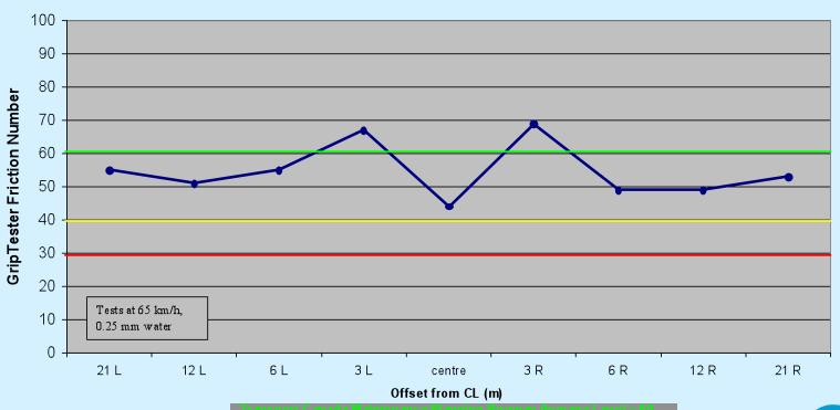
Transport Canada Maintenance Planning Runway Average Level = 60 Transport Canada Minimum 100 m Maintenance Planning Level = 40 Transport Canada Minimum 100m Action Level = 30
