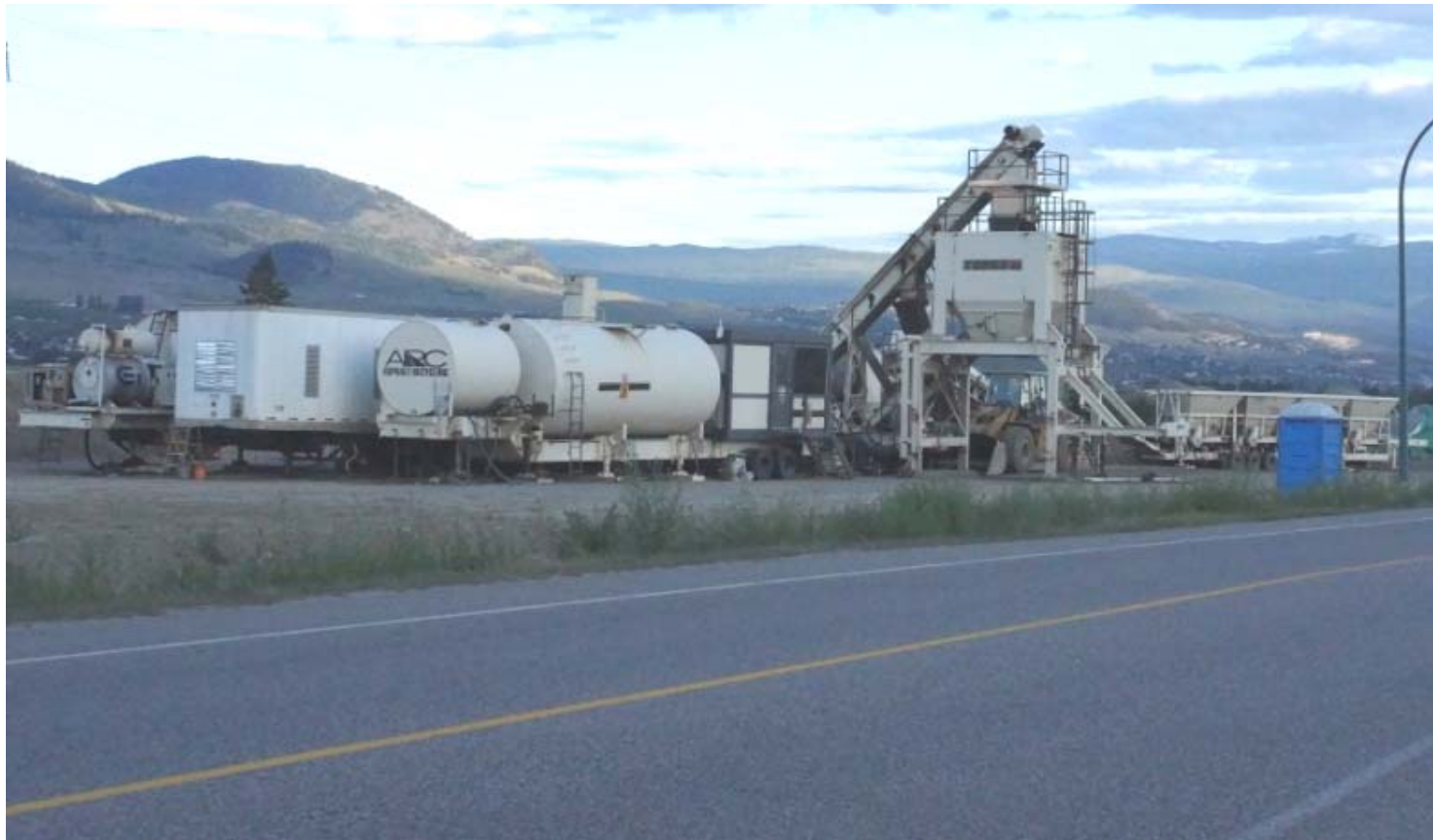
ARC's on site, Terex 150 TPH, Portable Drum Mix Asphalt Plant, ~ 1 km from airport
