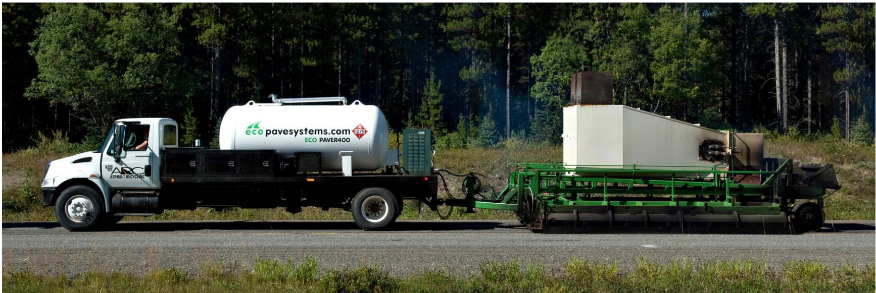
ARC's Ecopaver 400 pre-heater (two versus the usual one)
