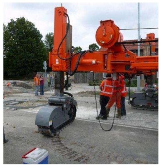
Designed to Rapidly and Semi-automatically Walk into the Transport Position
