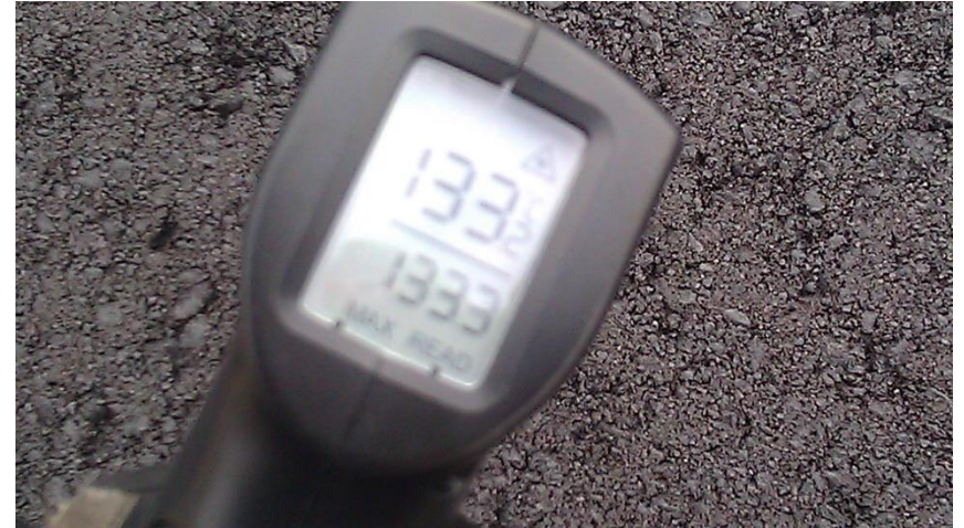
Checking asphalt compaction temperature on each subsequent asphalt layer
