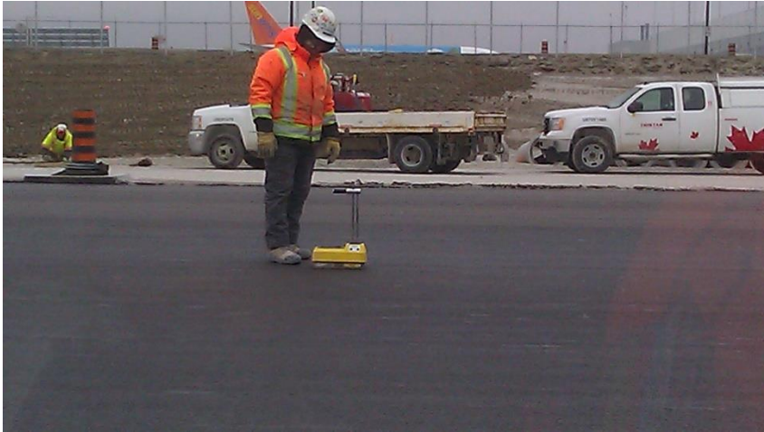
Checking in-situ asphalt density on each subsequent asphalt layer using nuclear gauge
