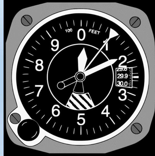
Aircraft altimeter displaying an altitude of 10,180 feet.
