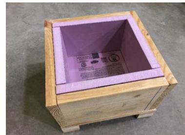
Mold with Thermal Insulation
