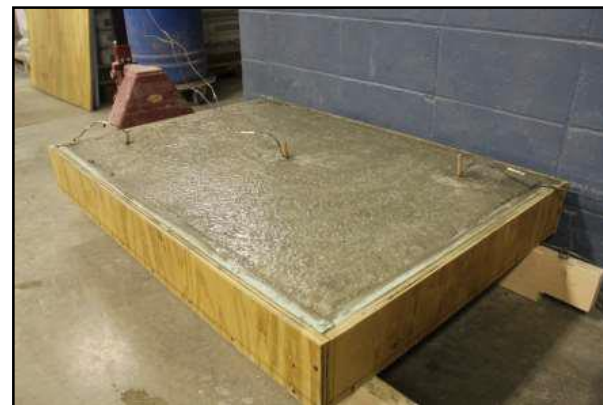
Completed ECON Test Slab
