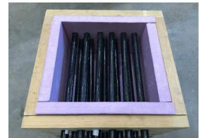
Mold with Embedded Pipes
