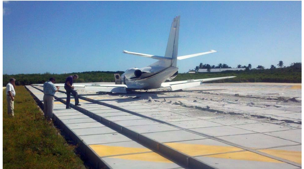
Source: Key West International Airport, 2011. Cessna Citation brake failure after landing
