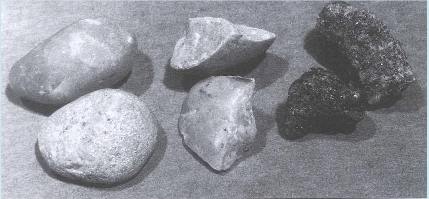
Figure 2.24 Aggregate of Various Shapes and Surface Textures
