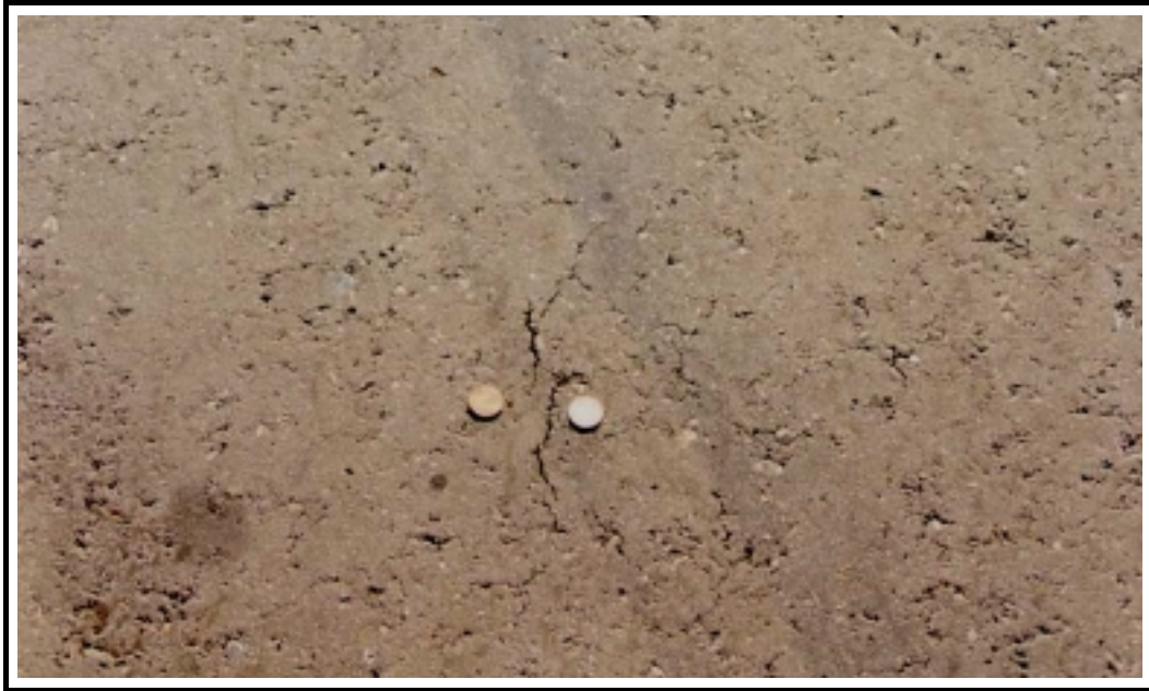
Photo 1 Very minor crack in PG Binder Test Section (~2+050) - September 1999
