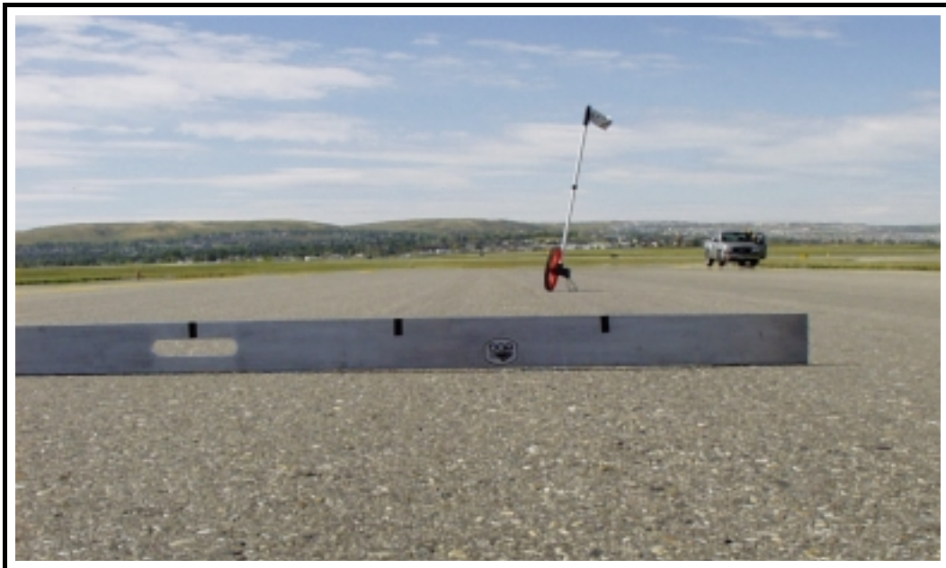
Photo 6 Very minor depression along longitudinal joint with low severity ravelling/weathering in PG Test Section - September 2000
