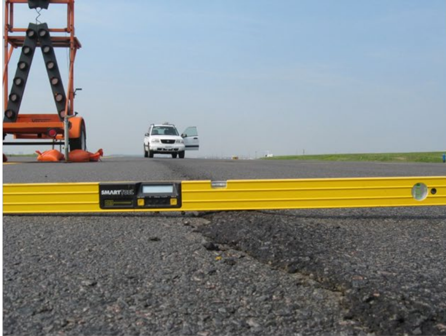
Asphalt Sliding between layers due to braking and turning
