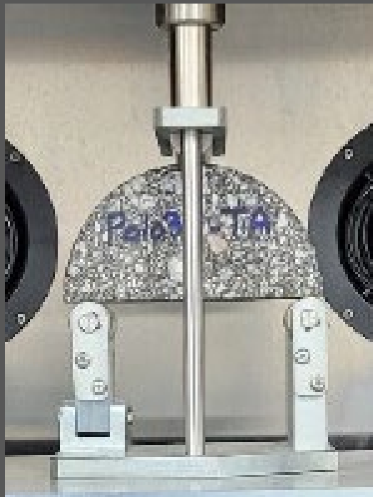
Semi Circular Bend (SCB) Test Fatigue Index at 25°C
