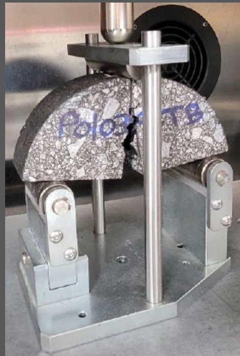
Semi Circular Bend (SCB) Test Fatigue Index at 25°C
