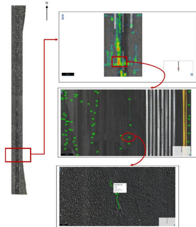
Example of Cracking Defects-2mm GSD
