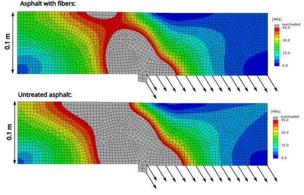
Von Misses stress contour plot could be used to identify overloaded areas.
