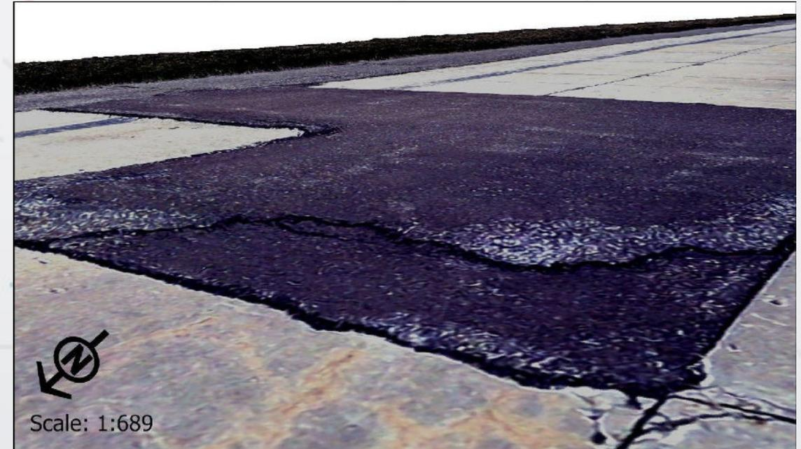
Example of draping an sUAS-derived Orthophoto over a DEM showing elevation differences for patching on airport runway
