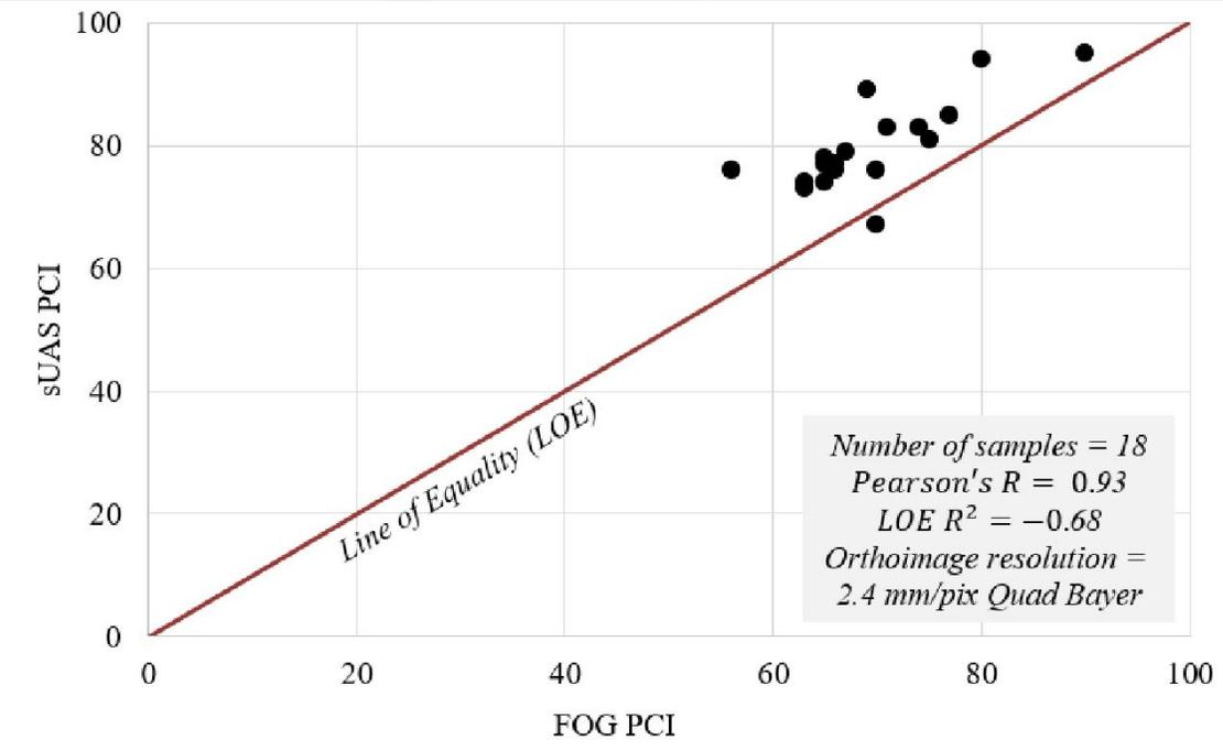
Comparison Between FOG PCI and sUAS PCI Calculated Using 2.4-mm/pix Data from TTF
