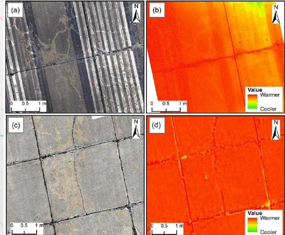
LTD Cracks and D-cracks in PCC Pavement on Runway 17/35 at ONZ
