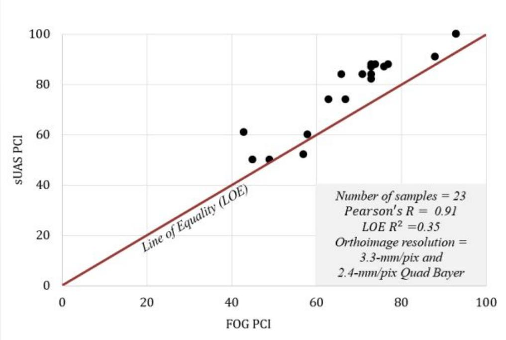
Comparison Between FOG PCI and sUAS PCI Calculated Using 2.4-mm/pix and 3.3-mm/pix Data from BNW
