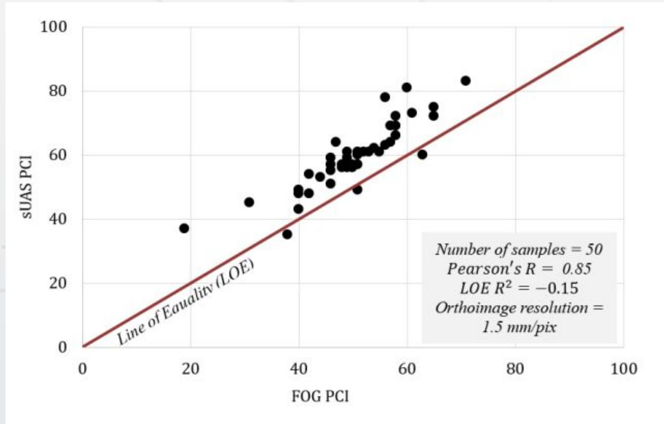
Comparison Between FOG PCI and sUAS PCI Calculated Using 1.5-mm/pix Data from WWD
