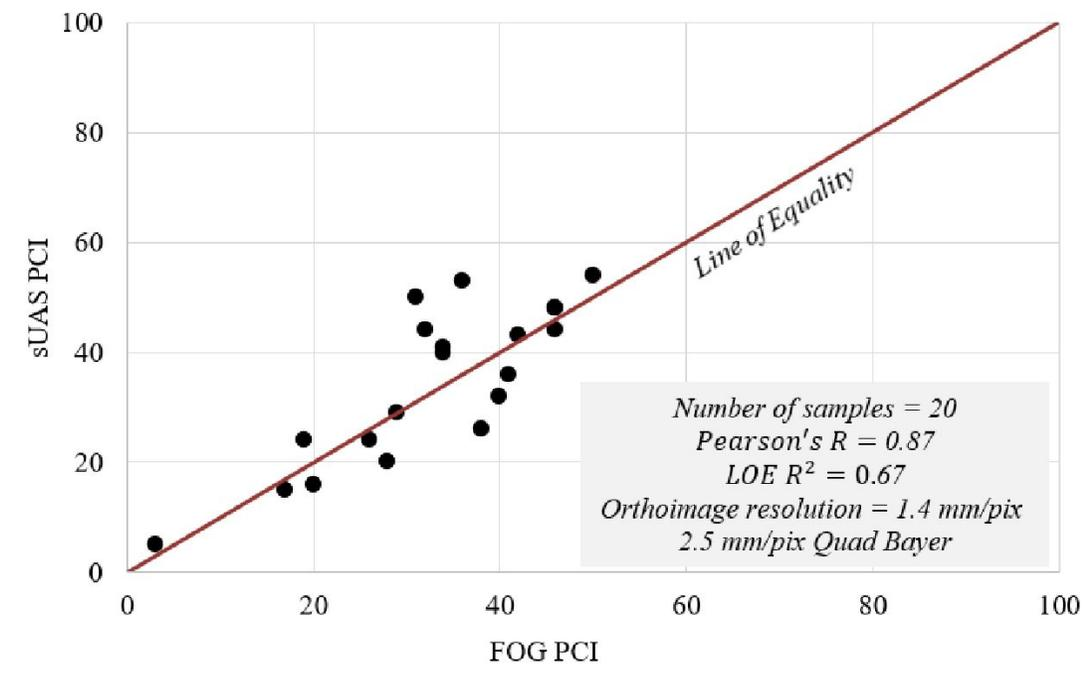
Comparison Between FOG PCI and sUAS PCI Calculated Using 1.4-mm/pix and 2.5-mm/pix Data from ONZ
