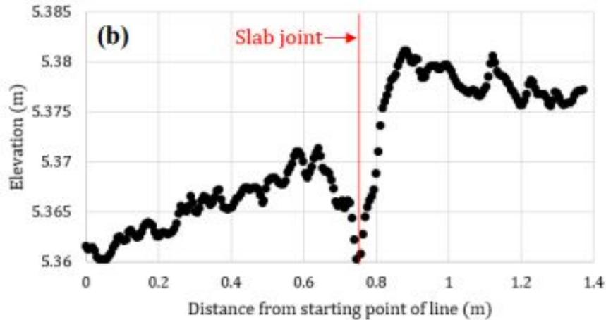
3D profile of pavement with Faulting (M)
