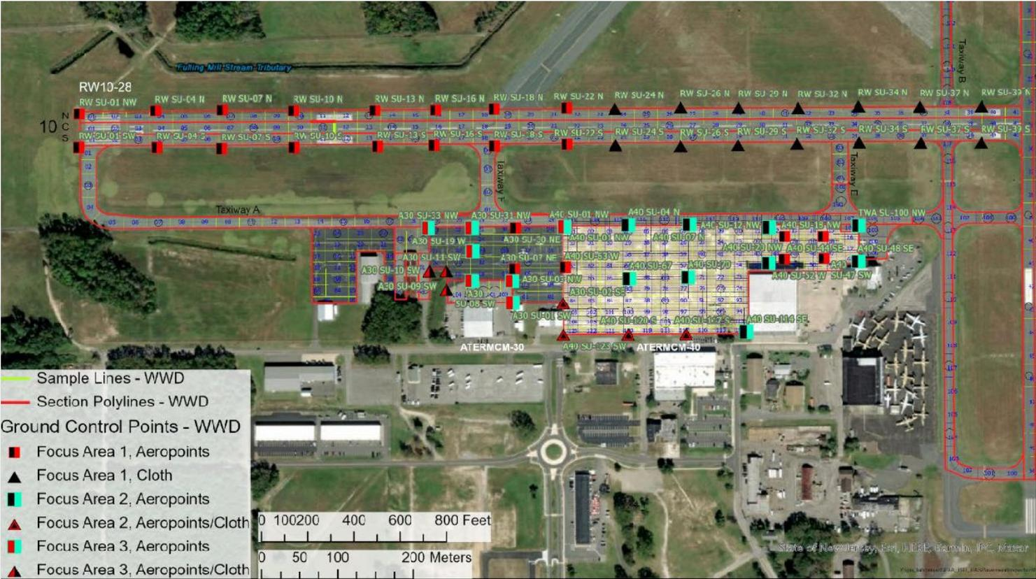
Ground Control Point locations planned at WWD spaced at 100-m intervals
