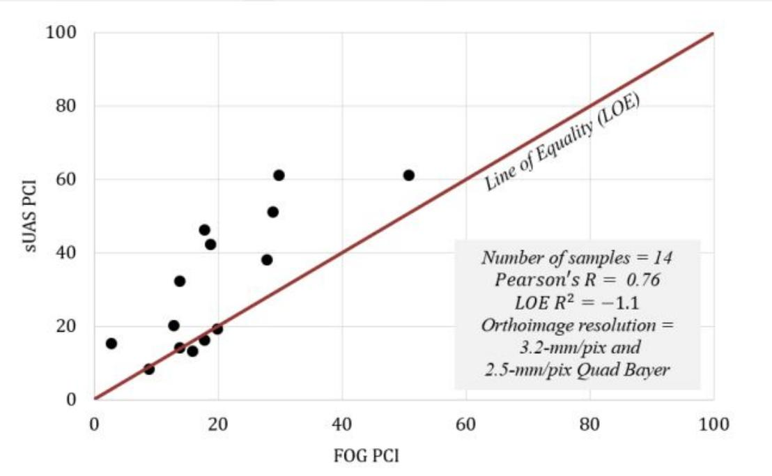
Comparison Between FOG PCI and sUAS PCI Calculated Using 2.5-mm/pix and 3.2-mm/pix Data from PRO
