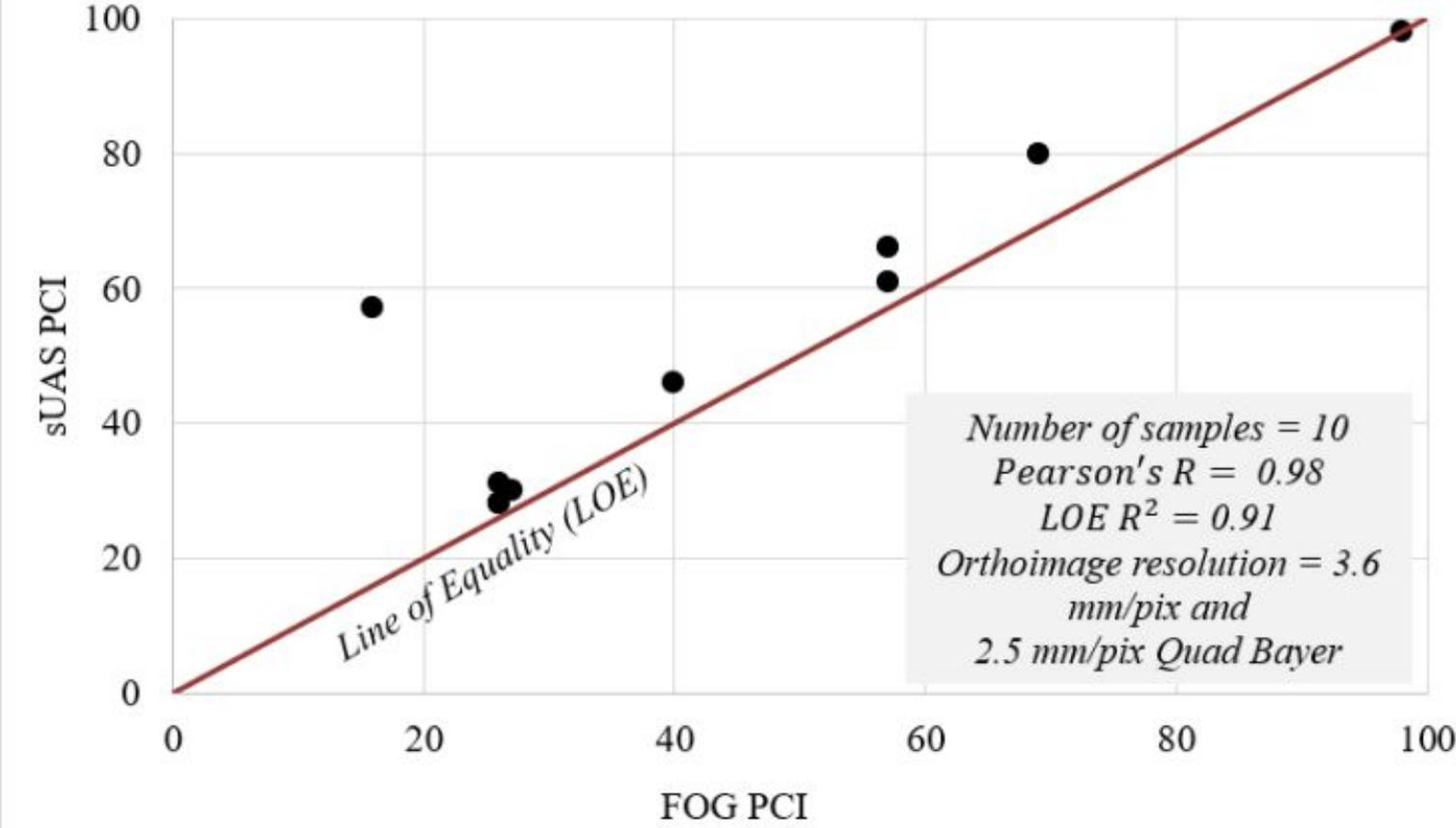
Comparison Between FOG PCI and sUAS PCI Calculated Using 2.5-mm/pix and 3.6-mm/pix Data from MTO
